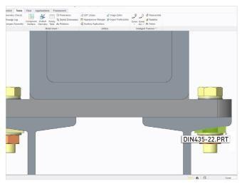
Automatically orientate wedge washers during placement
