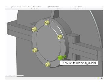
Assemble fasteners on all instances
